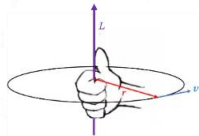
Suppose the image above is tilted upward to resemble the pitcher's arc path while throwing the ball, as shown in the first image below. In this case, if we use the right-hand rule, the angular momentum  $L$  points into the paper where the radius  $r$  is
