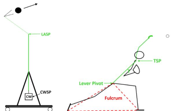
As mentioned earlier, perfect vertical alignment of the  $L_1$ ,  $L_2$ , and CW and optimal LASP and CWSP enhance the distance and velocity of a projectile launched from a trebuchet. The conservation of energy
